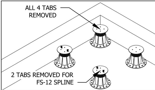
1. PLACE PEDESTALS AROUND PERIMETER AND REMOVE TABS AS NECESSARY.
