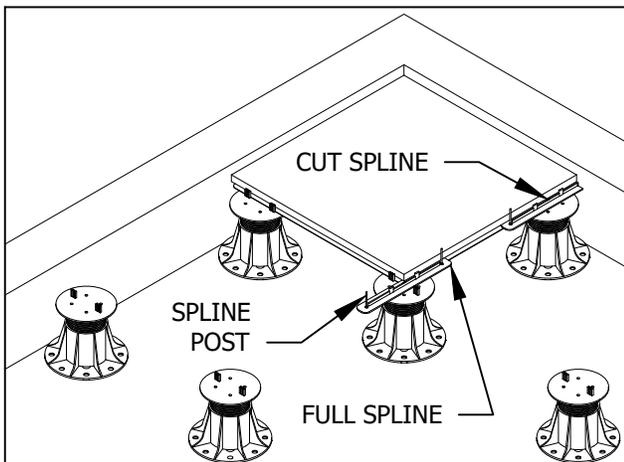
3. USING THE SPLINE POSTS, SLIDE FS-12 SPLINES INTO CHANNEL OVER PEDESTALS. PERIMETER SPLINES IN LINE WITH TRAY CHANNEL SHOULD BE CUT DOWN WITH A SAW AS NEEDED IN ORDER TO CENTER OVER EACH PEDESTAL.
