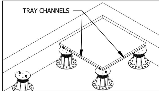
2. PLACE PAVER TRAY ASSEMBLY ON TOP OF PEDESTALS.
