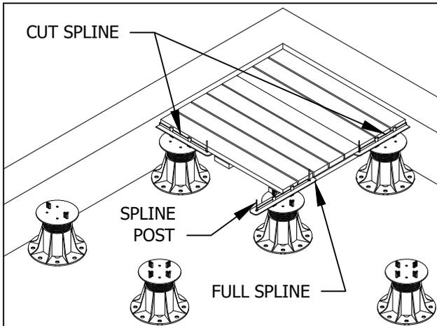
3. USING THE SPLINE POSTS, SLIDE FS-12 SPLINES INTO WOOD TILE KERF OVER PEDESTALS. PERIMETER SPLINES SHOULD BE CUT DOWN WITH A SAW AS NEEDED IN ORDER TO CENTER OVER EACH PEDESTAL.
