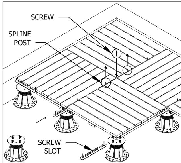
4. SCREW SPLINES INTO CENTER OF PEDESTAL TOPS, AND REMOVE POSTS WITH PLIERS, TAKING CARE NOT TO DAMAGE THE WOOD TILES. (DO NOT ATTEMPT TO HAMMER THE POSTS)
