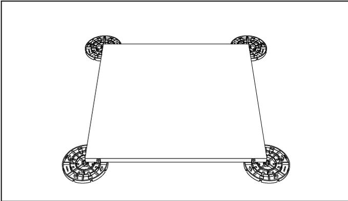
1. PLACE PAVER FINISH FACE DOWN OVER FOUR (4x) PEDESTALS AS SHOWN. PULL PAVERS FROM DIFFERENT BOXES AND / OR PALLETS IN ORDER TO ACHIEVE AN EVEN COLOR DISTRIBUTION.
