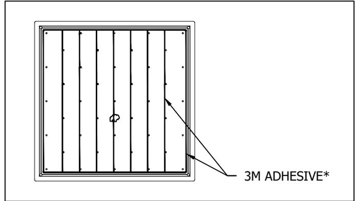
2. RUN A 1/8" DIA. BEAD OF PROVIDED 3M ADHESIVE, OFFSET 1/4" FROM THE TOP OUTER EDGE OF THE TRAY, AND A 1/8" DIA. BEAD ALONGSIDE EACH LINE OF HOLES AS SHOWN. \*IMPORTANT: FOR PROPER ADHESION AND PERFORMANCE, ADHESIVE MUST BE APPLIED EXACTLY AS SHOWN. TO PREVENT MOISTURE FROM ENTERING BETWEEN PAVER AND TRAY, A CONTINUOUS PERIMETER BEAD OF ADHESIVE MUST BE INSTALLED ALONG THE EDGE OF THE TRAY.
