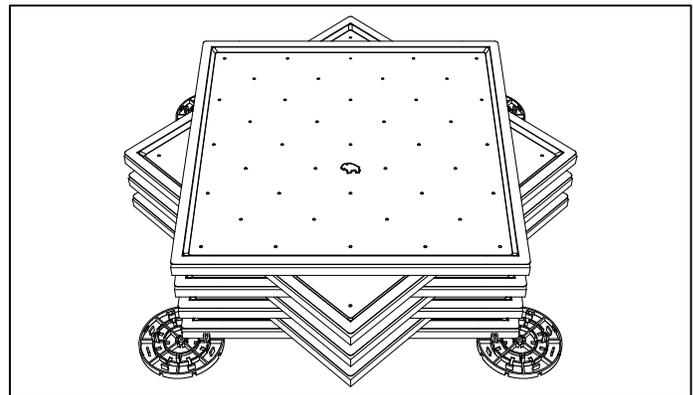
4. REPEATING THE FIRST THREE STEPS, GENTLY LAY EACH NEW PAVER ON TOP OF THE PREVIOUS TRAY, ROTATING AS SHOWN. STACK NO MORE THAN TEN (10x) PAVERS HIGH, AND LET THEM SIT FOR 2 TO 4 HOURS, OR UNTIL THE ADHESIVE HAS CURED, BEFORE HANDLING.
