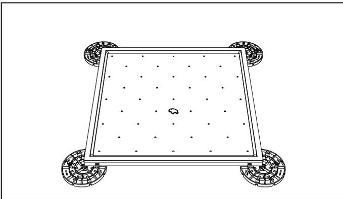
3. PLACE THE ADHESIVE SIDE OF THE TRAY SQUARELY ONTO THE PAVER, CAREFULLY ALIGNING BY HAND TO MAKE SURE THAT THE TRAY DOES NOT EXTEND BEYOND ANY EDGE OF THE PAVER.
