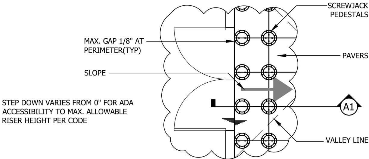
STEP DOWN VARIES FROM 0" FOR ADA ACCESSIBILITY TO MAX. ALLOWABLE RISER HEIGHT PER CODE
