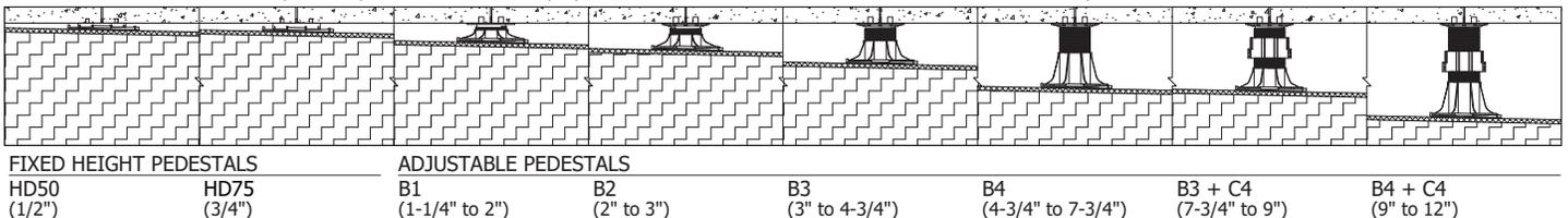
NOTE: Pedestals each shown with one optional LD4 slope compensation accessory.
