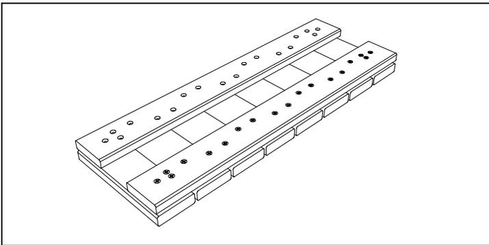
3. USING THE BOTTOM RUNNER REMOVED IN STEP 2 TO ALIGN THE HOLES, PRE-DRILL ACCORDINGLY WITH A CARBIDE BIT ON THE PORTION TO BE INSTALLED. BE SURE TO MAINTAIN A CONSISTENT SPACING BETWEEN THE PLANKS.
