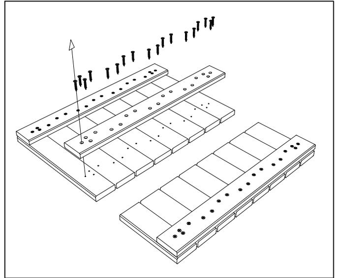
2. AFTER CUTTING, WITH THE TILE UPSIDE DOWN, REMOVE A BOTTOM RUNNER FROM THE PORTION TO BE DISCARDED, BEING CAREFUL TO NOT STRIP THE SCREW HEADS.
