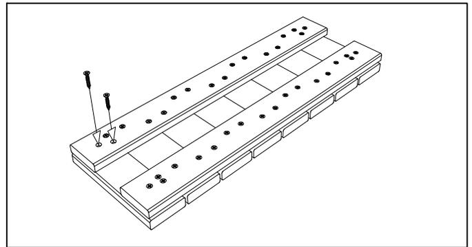
4. AFTER PRE-DRILLING, SCREW THE RUNNER INTO PLACE ON THE PORTION TO BE INSTALLED, RE-USING THE SCREWS REMOVED IN STEP 2.
