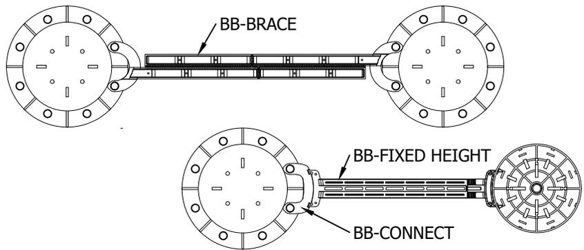
4. LOCK THE BRACING ARMS TOGETHER BY INSERTING BB-LATCHES INTO THE SIDE OF EACH BISON BRACE OR BB-SCREWS INTO THE TOP OF EACH BB-FIXED HEIGHT, AND TWIST 90 DEGREES.
