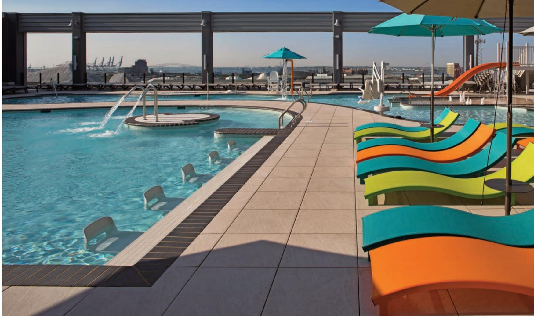
**Bison 2CM Pavers are a beautiful surfacing option for rooftop environments.** Available with a wood, stone, or concrete appearance, Bison 2CM Pavers create aesthetic appeal for rooftop decks, outdoor areas, or pool surrounds. Must be used with the Bison Paver Tray or Backer when installed over Bison Pedestals.
